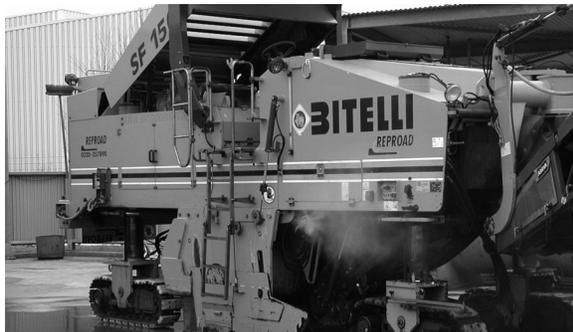
Figure 2. Asphalt milling machine equipped with new dust emission reduction system.
