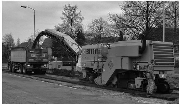
Figure 1. Asphalt milling machine (Bitelli SF202)
