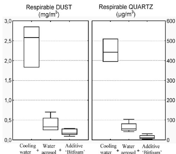
Figure 3. Box-plot (min-25%-median-75%-max) of the measured concentrations of respirable dust and crystalline quartz in the breathing zone of operators of a asphalt milling machine equipped with: (i) only a cooling water system (standard), (ii) a system of spraying water aerosol, and (iii) a system of spraying water aerosol with the additive Bitfoam.
